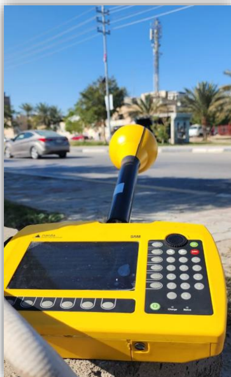
Fig. 4: Placing the device Narda SRM 3006 and directing the probe on the tower to take measurements.
