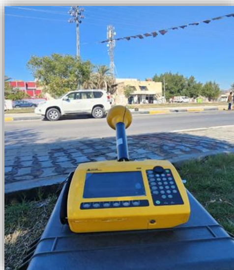
Fig. 2. Narda SRM 3006 Measuring system and Location of the measuring point.
