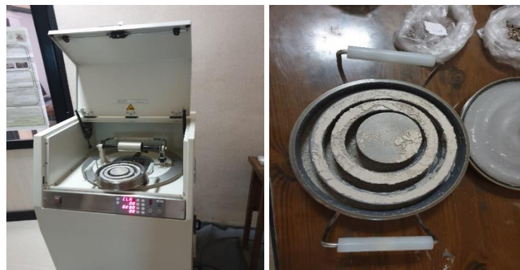
Figure 2. Disc vibrator and its lining.
