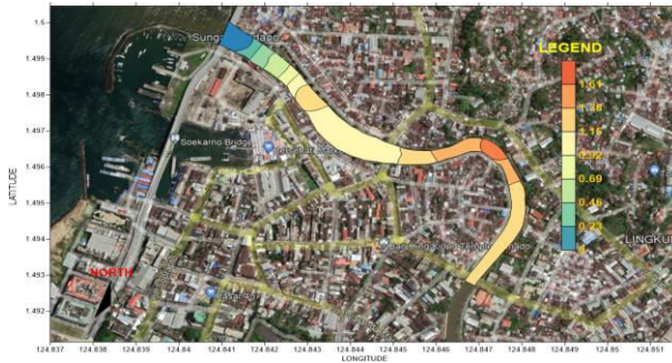
Figure-1. Map of the mass flow density model at high tide Muara Kuala Jengki Manado
